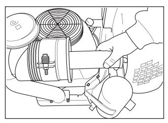
Removing the inner filter
